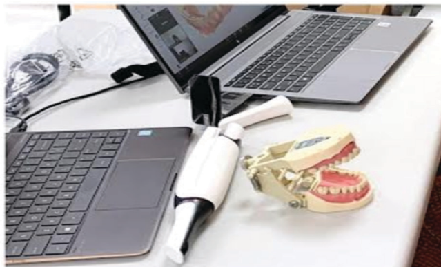
Figure 1.2: The TRIOS 4 intraoral scanner (3 shape A/S), which uses confocal technology and enables integration with CAD software programs and CAM devices from other manufacturers.
