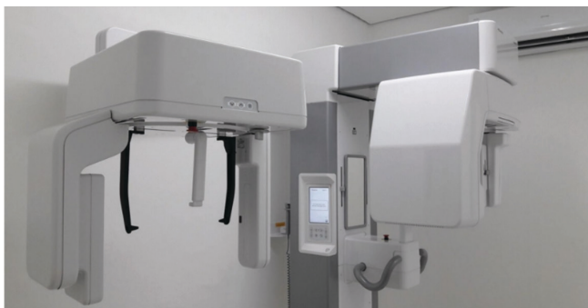
Figure 2.1: A CBCT device integrated with cephalometric and panoramic radiographic functions (Cranex 3D, Soredex, Tuusula, Finland)
